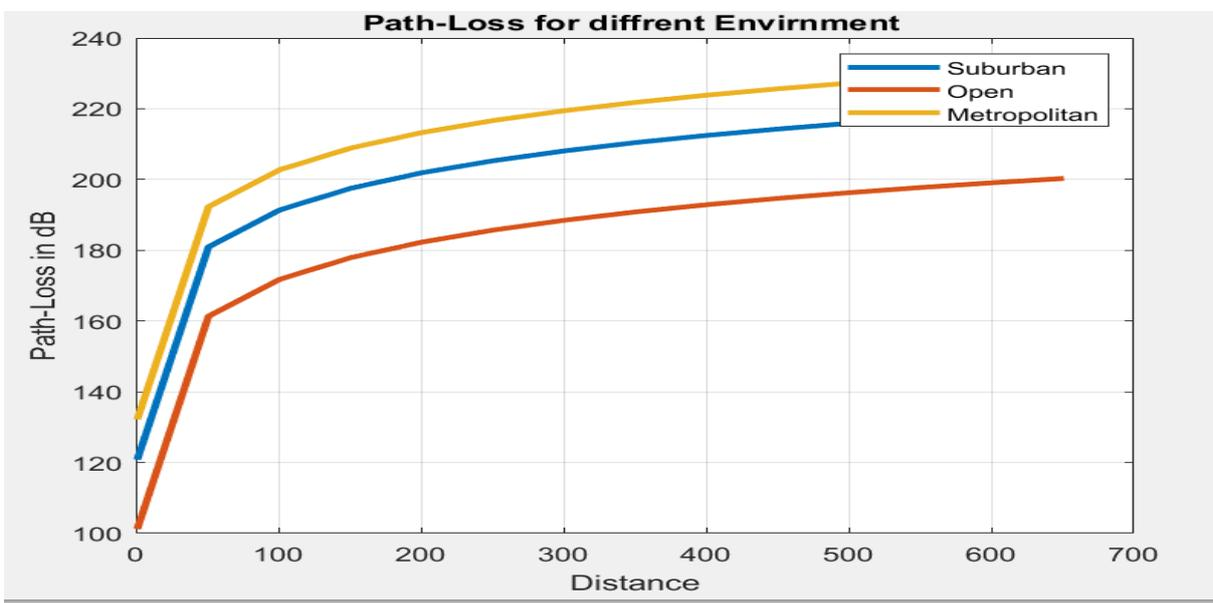
Figure 13 Okumura Hata Model (700 km span for different environments)
