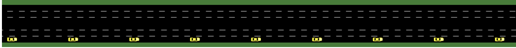
Figure 5.9: The result of speed harmonisation with a streamlined flow of vehicles on a lane
