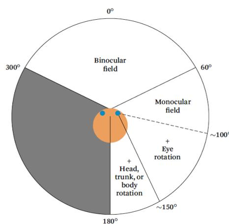
Figure 7: Horizontal FOV with straight ahead fixation, maximum lateral eye rotation and head rotation
