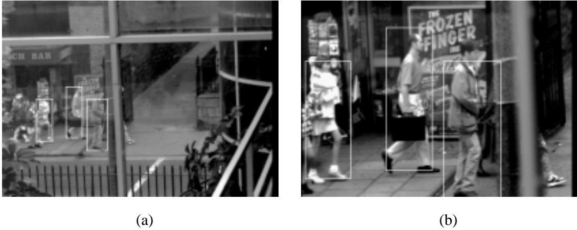
Figure 1: Wide angle (a) and zoomed (b) camera views showing the tracked objects marked with rectangles.
