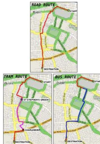
Fig. 6. Multi-modal journeys produced by STIS, and displayed using the stand-alone GUI client. All routes have identical start and destination points, but differ in the preferred modes of transport used when planning each route.
