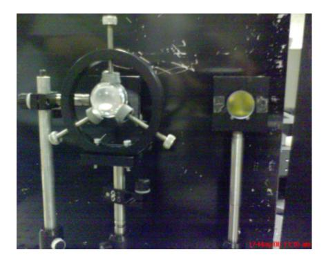
Fig. 4.5: Two reflector targets
