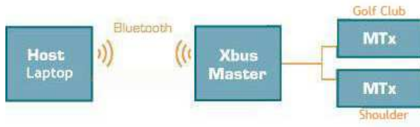
Figure 3.8: The Hardware Design View
