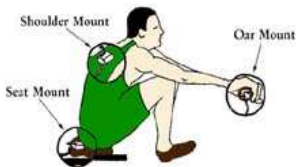
Figure 2.1: Accelerometer placement in experiments
