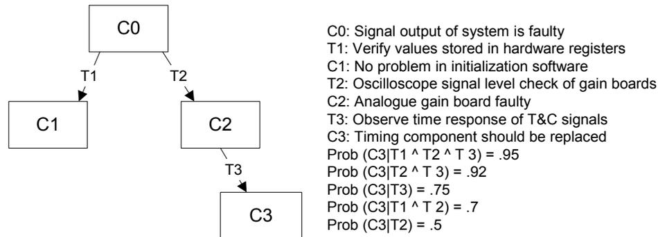
**Figure 3:** Example reasoning of digital signal processing expert system (Wolverton, 1995)
