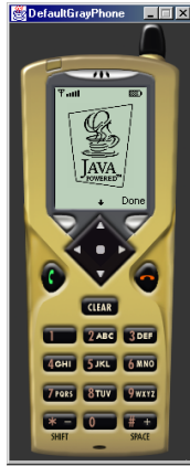
Figure 2.2: A J2ME MIDP application running on a cellular telephone emulator
