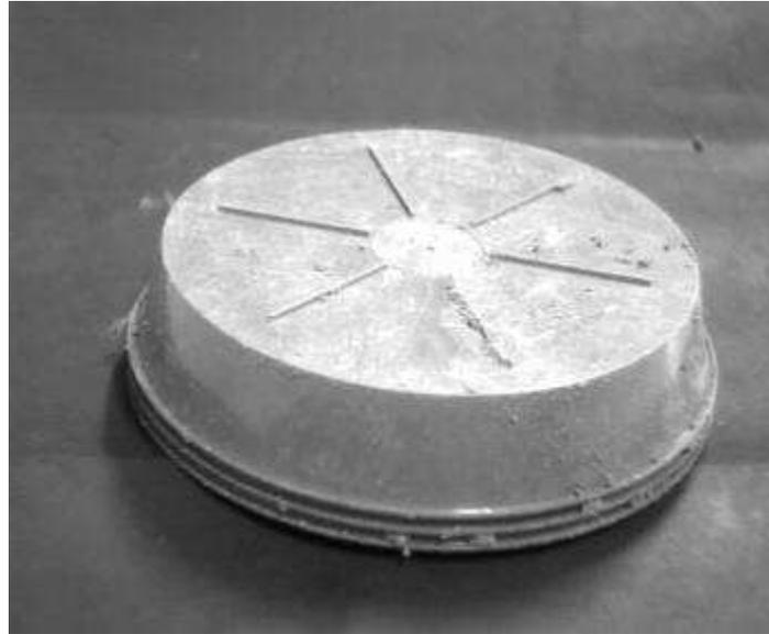
Figure 4: The simulated plastic anti-personnel mine
