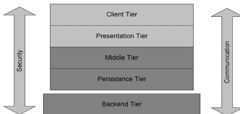
Figure 2. Structural view of e-government applications - a four tier architecture (SAGA, 2003)
