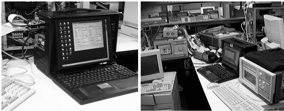
Figure 2: left: tracer/analyzer for the Scalable Coherent Interconnect (SCI), and right: in a heavily instrumented environment (see http://www.cs.tcd.ie/coghlan/scieuro/ ).
