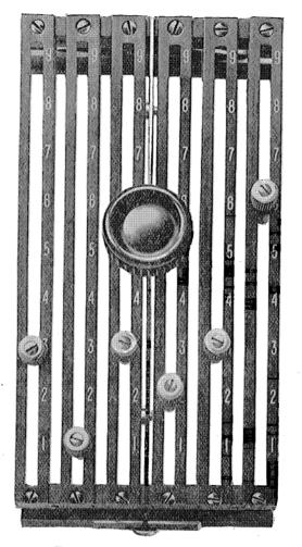
FIG. 3.—The Multiplying Device.
