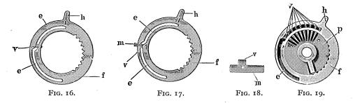
The pin wheels shown in fig. 13, whose adjustable pins m (figs. 17 and 18) are set by the lever h, are mounted on a common shaft worked by a crank. There are nine pins which can be made to project from the pin wheel as required, and when the crank is turned to rotate the shaft, these pins gear with small toothed wheels  $i^1$ ,  $i^2$  (figs. 20 and 21), which in turn gear with the number wheels E.
