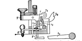
FIG. 49.-(<sup>2</sup>/<sub>3</sub> actual size.) Displacement of carriage (side view).
