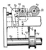
**FIG.** 50.—( $\frac{2}{3}$  actual size.) Last carriage axle with fittings for automatic check (front view).
