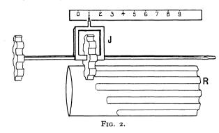
be increased to six. When the handle H has been adjusted the wheel is turned as a whole, and the knobs K knock the counter as they pass it.
