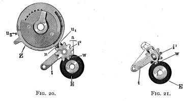
The pin w of the number wheel E displaces the hammer-shaped lever t (fig. 21) in such a way that the laterally movable pin  $u_1$  (fig. 20) on the pin wheel Z engages with the next toothed wheel  $i^2$  and moves this one tooth forward.
