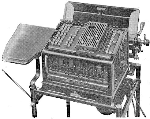
FIG. 2.—The Keyboard, showing the Multiplying Device.
