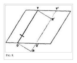
Next let the rod be moved parallel to itself, but in a direction not perpendicular to itself (fig. 8). The wheel will now not simply roll. Consider a *small* motion of the rod from QT to Q'T'. This may be resolved into the motion to RR' perpendicular to the rod, whereby the rectangle QTR'R is generated, and the sliding of the rod along itself from RR' to Q'T'. During this second step no area will be generated.
