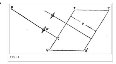
planimeters are made either with a rod QT of fixed length, which gives the area therefore in terms of a fixed unit, say in square inches, or else the rod can be moved in a sleeve to which the arm OQ is hinged (fig. 13). This makes it possible to change the
