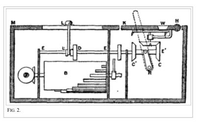
the window. This motion of all the wheels C is done simultaneously by the push of a lever which appears at the top plate of the machine, its two positions being marked "addition" and "subtraction." The B-wheels are in fixed positions below the plate MK. Level with this, but separate, is the plate KH with the window. On it the figure disks are mounted.
