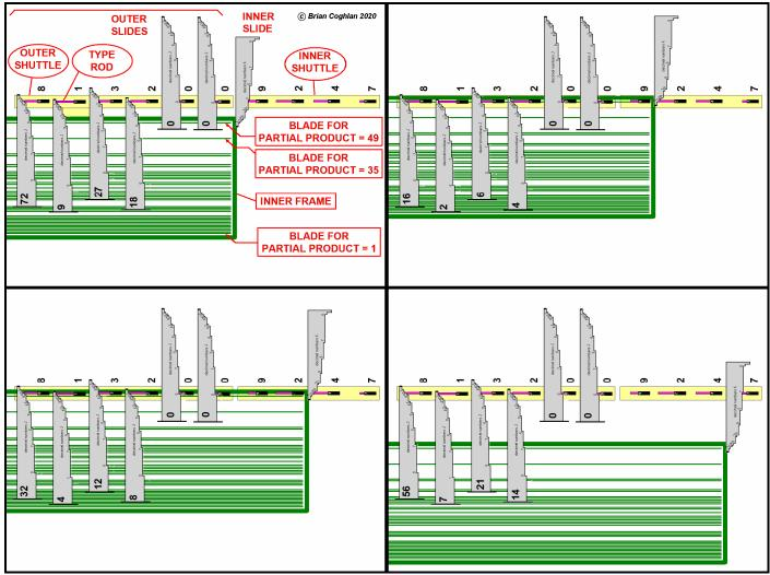
Figure 13 Ludgate's procedure for multiplication of two operands,
