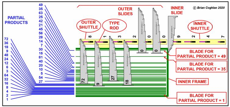
Figure 12 Ludgate's outer and inner logarithmic index slides, and inner frame with blades for compound indexes, representing the machine with a 6-digit outer operand and a 4-digit inner operand as per Engineering [32] Note that the slides and shuttles will actually face directly away from the viewer, but are shown as is to aid understanding Images reproduced courtesy The John Gabriel Byrne Computer Science Collection
