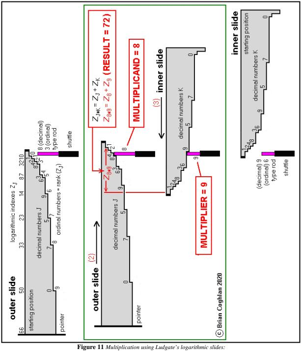
Left: outer slide at its starting position, Right: inner slide at its starting position, Middle: movement of slides for multiplication of 8\*9 = 72 Image reproduced courtesy The John Gabriel Byrne Computer Science Collection
