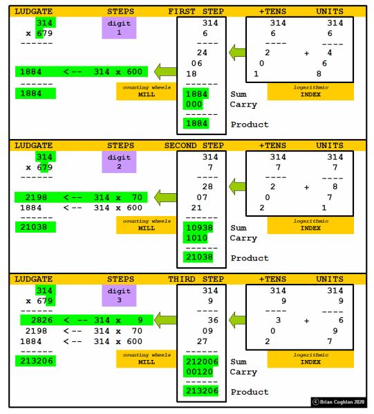
Figure 4 A possible order in which Ludgate's machine would have calculated 314×678 with one add and carries per stage. The right hand side shows how the partial products are split into tens and units Image reproduced courtesy The John Gabriel Byrne Computer Science Collection
