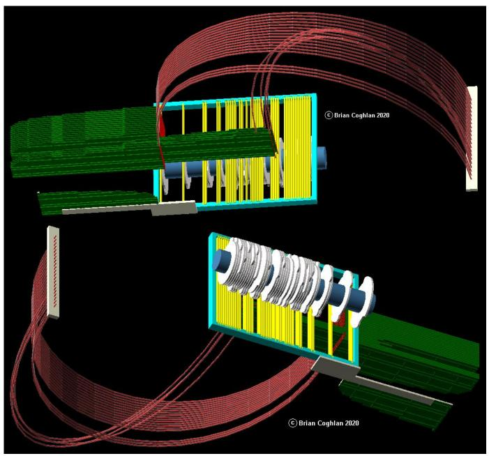
Figure 19 Early 3D renditions of a possible re-imagined Ludgate Index with flexible cables terminating in decimal-point carriage bar Images reproduced courtesy The John Gabriel Byrne Computer Science Collection
