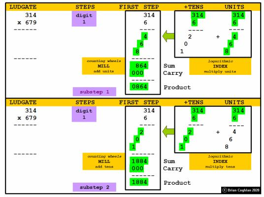
Figure 3 Ludgate's long multiplication steps for the multiplier MS digit. First multiply-accumulate units, then tens Image reproduced courtesy The John Gabriel Byrne Computer Science Collection
