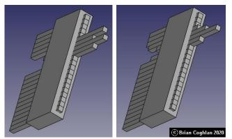
Figure 23 Speculative schematic of shuttles storing +813200.00 as ordinal +304199.99 (left) and +9167.00 as ordinal +6058.99 (right). The sign is the rod at the top, the next rod is the LS digit, and the bottom rod is the MS digit. The stored profiles are in reverse ranking of ordinals, see Table 4. The shuttle housing and rods are to correct scale but not representative in any other way.. Images reproduced courtesy The John Gabriel Byrne Computer Science Collection
