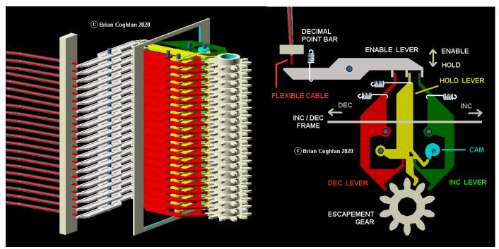
Figure 20 Speculative "conveyance mechanism using flexible cables to "enable" Mill wheel increment/decrement escapement TO BE DONE: The top layer of escapement levers (included as a placeholder) should be a sign management mechanism Image reproduced courtesy The John Gabriel Byrne Computer Science Collection
