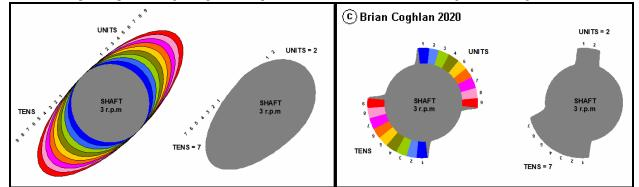
Figure 17 Left: Double-lobe cam with variable height raised segments (proportional to partial-product digit magnitude) over a fixed arc-angle Right: Double-lobe cam with fixed height raised segments over a variable arc-angle (proportional to partial-product digit magnitude) Image reproduced courtesy The John Gabriel Byrne Computer Science Collection
