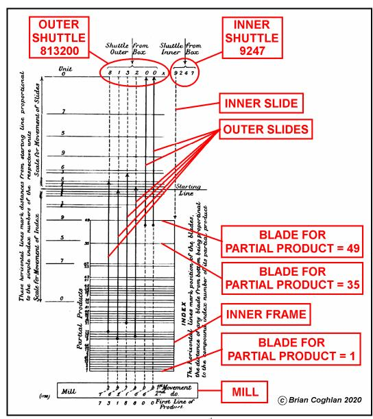
Figure 1 Annotated version of the diagram from Engineering, 20<sup>th</sup> Aug. 1909, Pages 256-257 [32] See Appendix I for the original full-size image Image reproduced courtesy The John Gabriel Byrne Computer Science Collection
