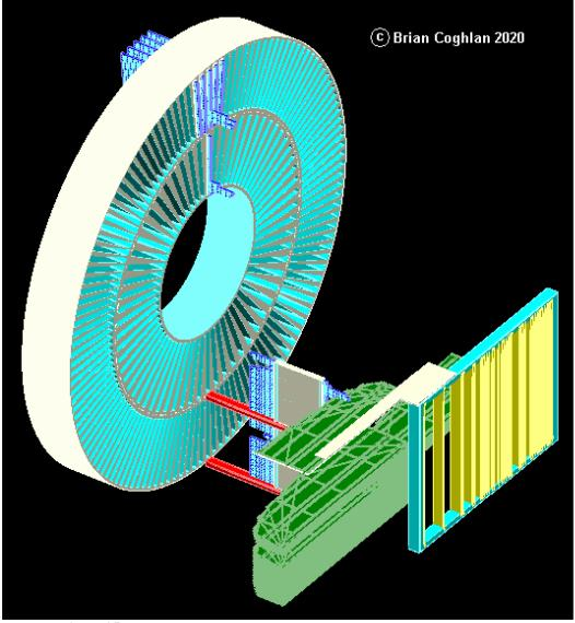
Figure 25 Early 3D rendition of a possible re-imagined Ludgate's storage and Index Three-quarter view showing inner and outer shuttles withdrawn along races Showing '813200' multiplied by '9247' as per Engineering [32] Image reproduced courtesy The John Gabriel Byrne Computer Science Collection
