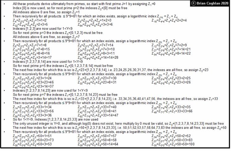
**Figure 6** Systematic method to derive Ludgate's index numbers **For all products** Y = (1 < J < 9) \* (1 < K < 9) **assign logarithmic index numbers**  $Z_Y = Z_{J^*K} = Z_J + Z_K$ Image reproduced courtesy The John Gabriel Byrne Computer Science Collection
