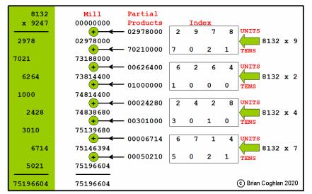
Figure 5 An example of Ludgate's variant of long multiplication, calculating 8132 x 9247 Image reproduced courtesy The John Gabriel Byrne Computer Science Collection
