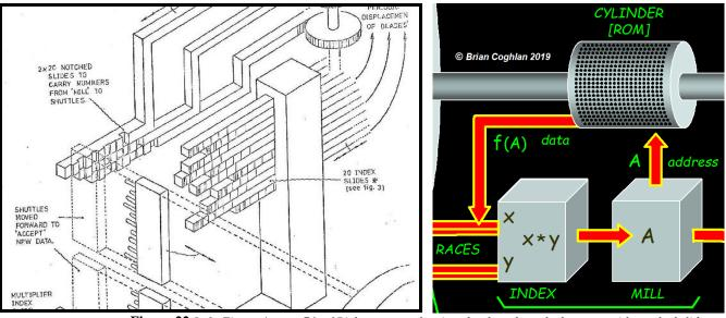
Figure 22 Left: Figure 4, page 76, of Riches report, showing shuttle rods pushed to mate with notched sliders Image reproduced courtesy Professor John Tucker, University College Swansea, UK Right: Conjectural diagram of path for cylinders to write ordinals to shuttles Image reproduced courtesy The John Gabriel Byrne Computer Science Collection
