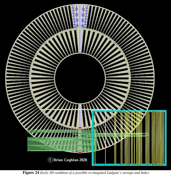
Figure 24 Early 3D rendition of a possible re-imagined Ludgate's storage and Index Top view showing alignment of storage cylinders and shuttles with Index with slides Showing '813200' multiplied by '9247' as per Engineering [32] Image reproduced courtesy The John Gabriel Byrne Computer Science Collection
