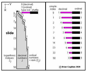
Figure 10 Re-oriented (left) Ludgate's logarithmic slide, (right) shuttle rod extensions for simple indexes, decimal and ordinal values Image reproduced courtesy The John Gabriel Byrne Computer Science Collection
