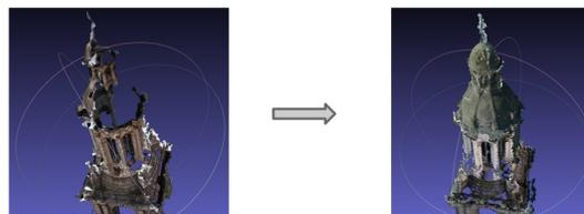
Figure 2: 3D reconstruction using additional visual information from drone images.
