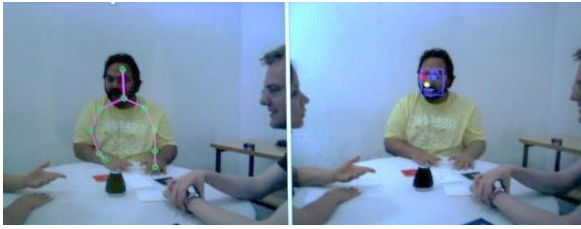
Figure 2: An overlay of the head pose and skeleton tracking by Kinect
