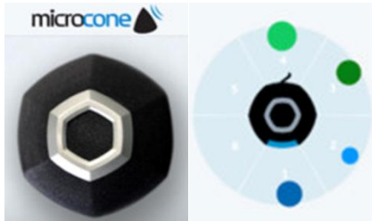
Figure 3: The Microcone® microphone array (left) and a visualization of an activity of the different microphones (right)
