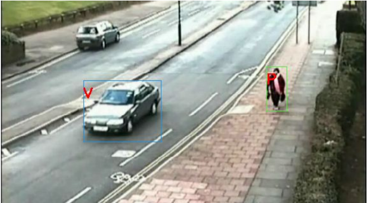
Figure 5.1: Correctly labelled car and pedestrian
