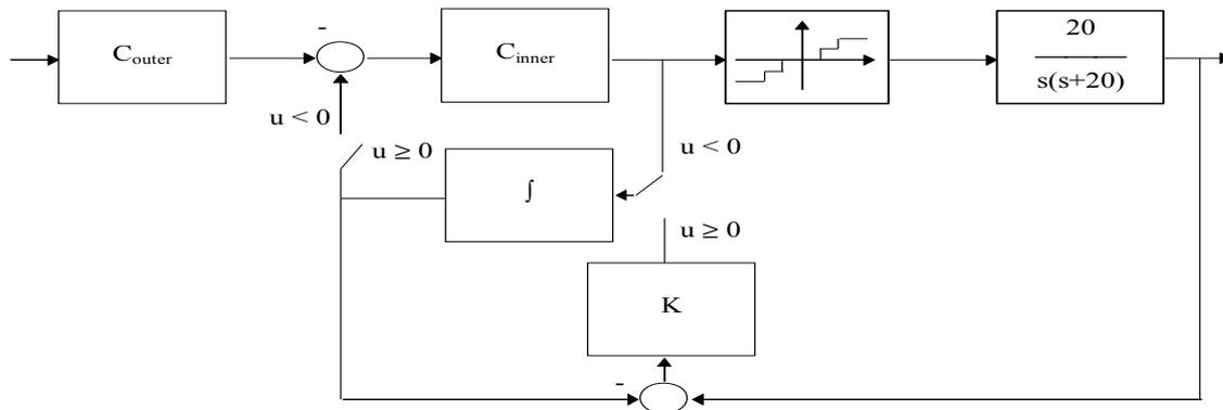
Fig 3 Arrangement employed for switching between below and above rated operation
