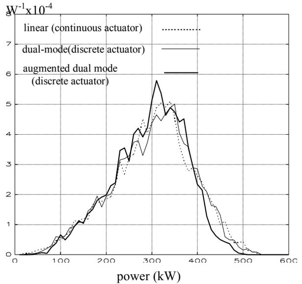
Fig 4 Probability density function of power (24 m/s wind, 20% turbulence intensity TI)
