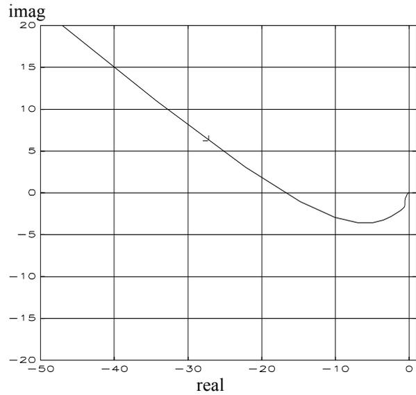
Fig 2 Nyquist plot of forward path transfer function
