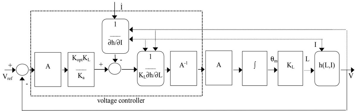
Figure 7 Gain-scheduled controller with feedforward<sup>2</sup>.
