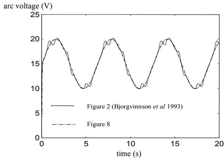
Figure 9 Simulated arc voltage responses for the control configurations of figure 2 and figure 6.
