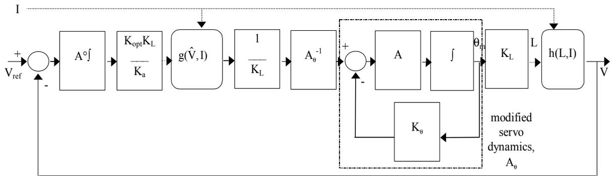
Figure 8 Reformulation of feedforward controller<sup>2</sup> which does not employ  $\dot{I}$ .
