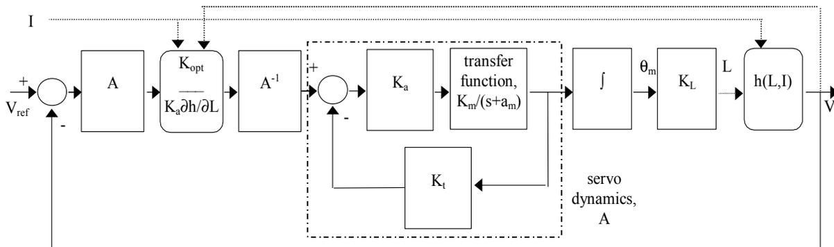
**Figure 5** Compensation for servo dynamics with scheduled gain positioned outside servo velocity feedback loop<sup>2</sup>.
