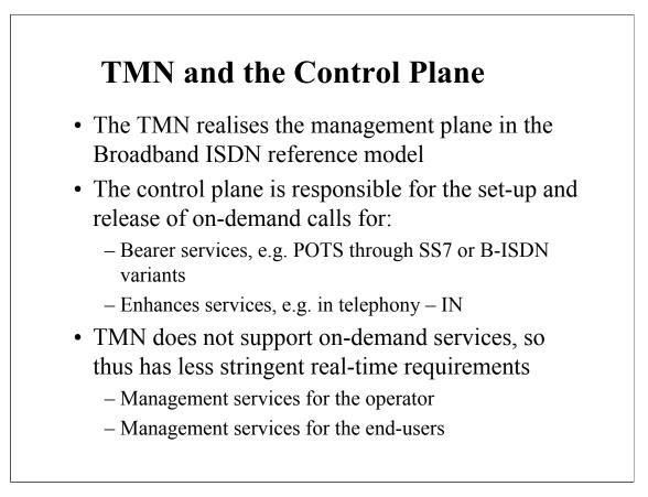
The distinction between the TMN and the telecommunications network it manages maps exactly to the distinction between the *management* and *control* planes of the Broadband ISDN Reference Model. The latter categorises activities into three *planes*:
