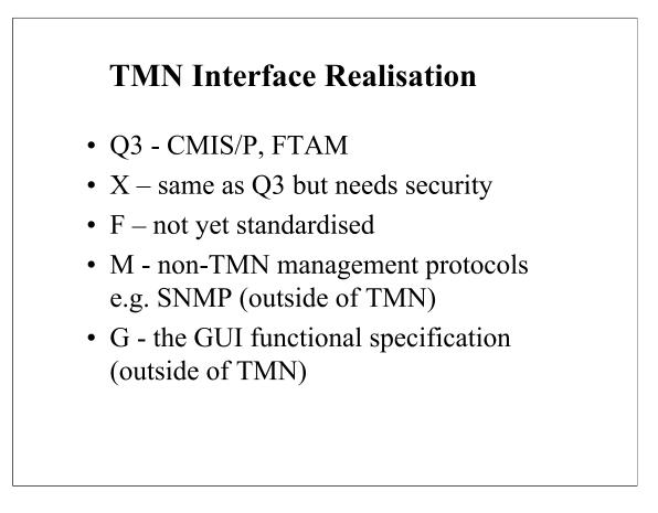
The TMN uses the OSI Systems Management standards wherever possible. This means that interfaces for intra- and inter-TMN communication are based on OSI management standards, with the exception of the F interface which may or may not have explicit management semantics.
