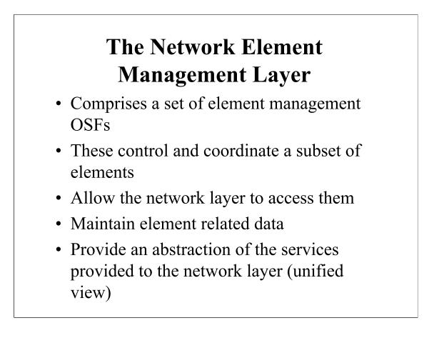
The element management layer manages each network element on an individual basis and supports an abstraction of the functions provided by it to the layer above i.e. the network management layer. It comprises a set of element management OSFs that are individually responsible on a devolved basis from the network management layer for a subset of network elements. Each such OSF has the following three major roles:
