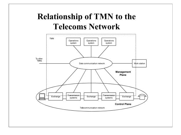
A TMN may provide management functions and offer communications between OSs themselves and between OSs and the various parts of the telecommunications network. The latter may consist of many types of analogue and digital telecommunications and support equipment, such as transmission and switching systems, multiplexers, signalling terminals, front-end processors, workstations, file servers etc. All this equipment is generically referred to in the TMN context as Network Elements (NEs).
