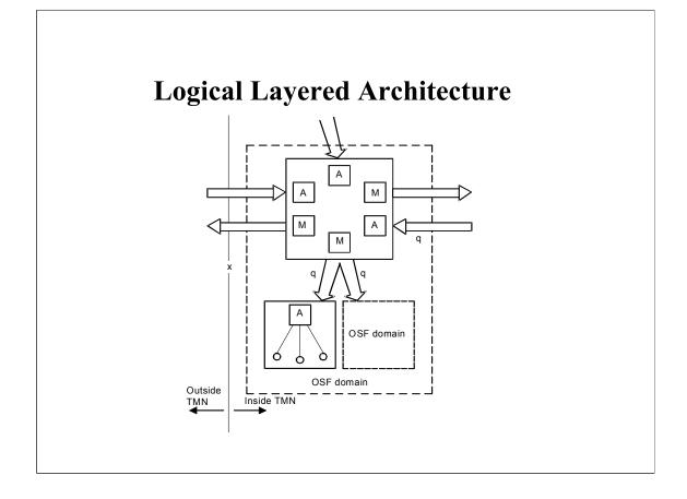
The Logical Layered Architecture (LLA) is a development concept based upon hierarchical design principles in which the architecture can be thought as being based on a series of layers. The scope of each layer is broader than the layer below it, more generic in functionality and its managed objects provide higher levels of abstraction e.g. services instead of transport connections.
