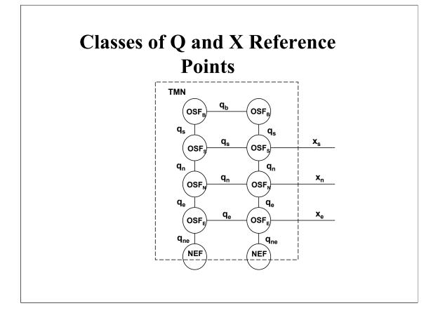
The TMN functional architecture defines generic classes of q and x reference points for management information exchange. Given the hierarchical decomposition of the TMN into element, network, service and business management layers, specific classes of those reference points can be defined between layers and within a layer. The figures depicts a hierarchical taxonomy of the relevant classes.
