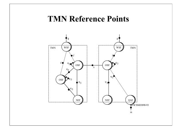
The TMN function blocks exchange management information through reference points. The latter are conceptual points and they only become interfaces when the connected function blocks are embodied in separate pieces of equipment. The key classes of TMN reference points are identified in the above figure.
