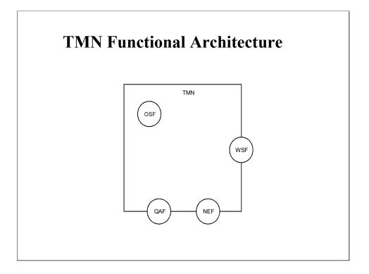
The TMN functional architecture is based on a number of function blocks which provide the TMN general functions. The overall functionality is broken down into two main components: the Operations System Function (OSF) and the Workstation Function (WS). A Network Element Function (NEF) and Q Adaptor Function (QAF) are also used to provide a view of the telecommunications network and services being managed.
