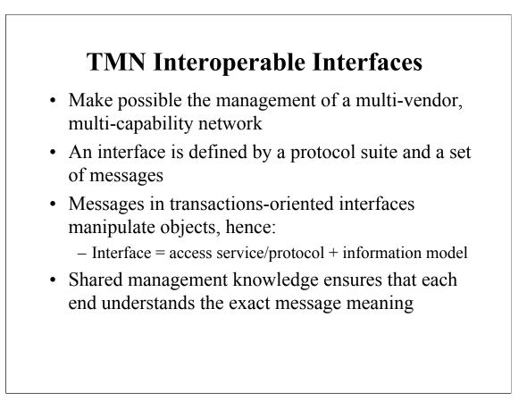
In order for two or more TMN building blocks to exchange management information they must be connected by a communications path and each element must support the same interface onto that communications path. Using the concept of an interoperable interface to simplify the communications problems arising from a multi-vendor, multi-capability network.
