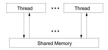
Multiple threads, but memory is still an array of values, or a sequentially consistent (SC) shared memory:
